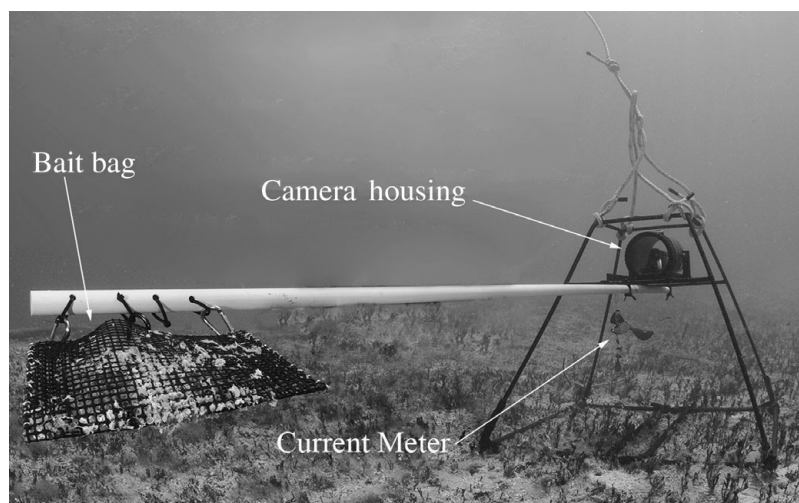
Fig. 2. Baited remote underwater video survey (BRUVS) unit deployed on the seabed
